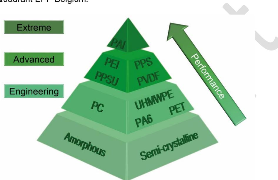
**Figure 1.** Thermoplastics provided by Quadrant EPP Belgium
